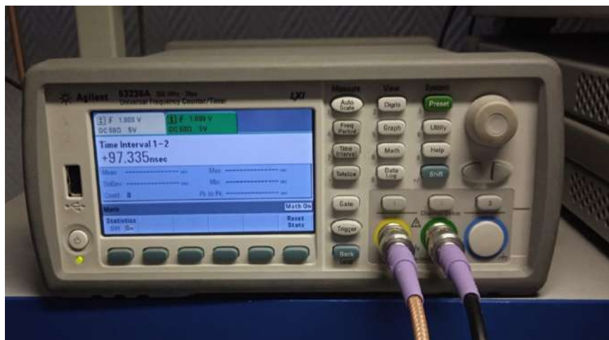
Fig. 2. Measuring the delay between the first and second pulses using an Agilent 53230A frequency counter
