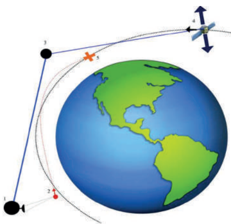
Fig. 1. Structural diagram of the network; 1 – AES detecting space debris; 2 – space debris; 3 – AES – participant of the mesh network; 4 – satellite threatened by the detected object; 5 – intersection of the debris trajectory and the orbit of the at-risk satellite
