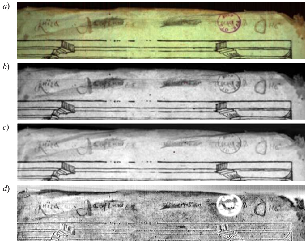
Fig. 3. Unreadable handwritten marginalia erased with ink. Original (a); UV light, band 480 nm (b); halogen lamp, light band 460 nm (c) UV light, PCA-4 (d)
