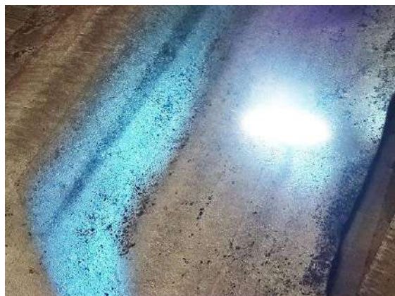
Fig. 3. Visual control of degree of laser cleaning
