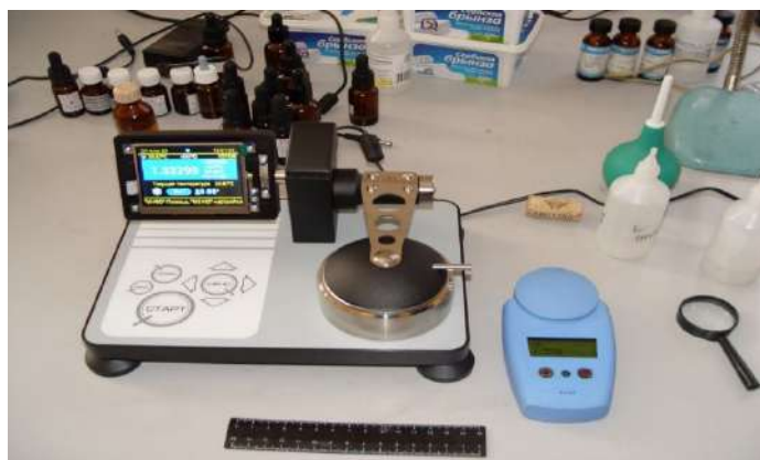
Fig. 1. Two refractometers: small-size and mobile (measuring distilled water)
