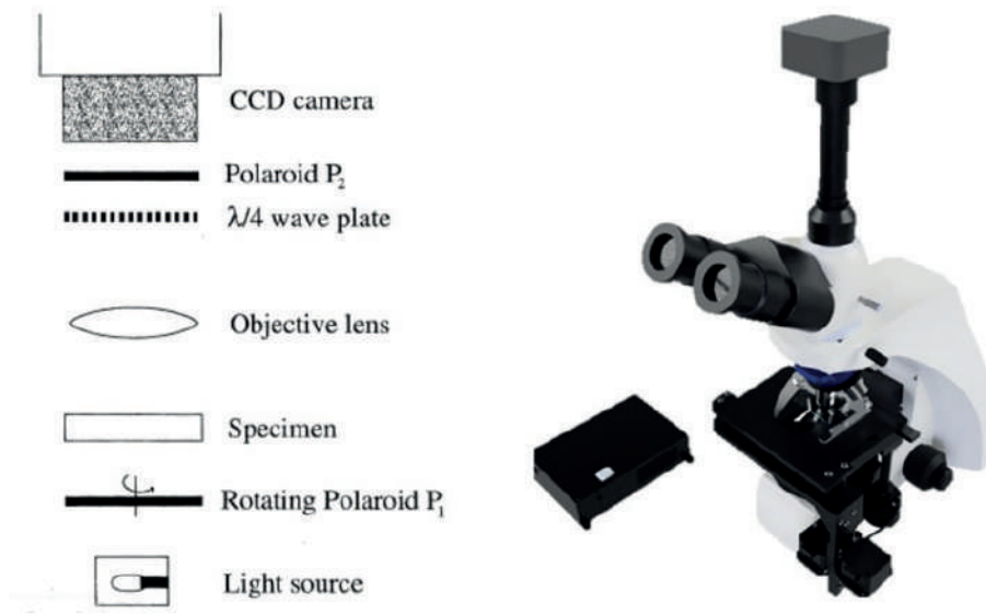
Fig. 1. The device and its optical scheme
