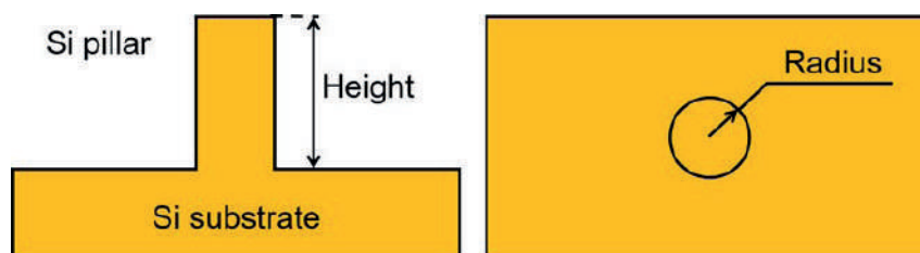
Fig. 1. Schematic of the single Si pillar for simulation
