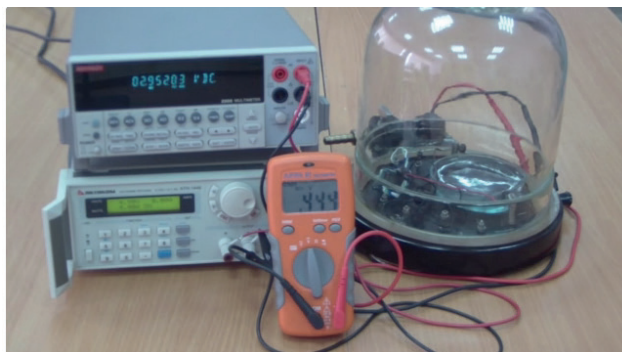
Fig. 2. Stand for measuring the output signal of the humidity sensor
