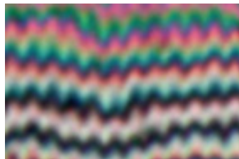
Fig. 8. Interferogram of relief profile for spatial frequency \nu = 550 \text{ mm}^{-1} (PFG-03M photographic plates)
