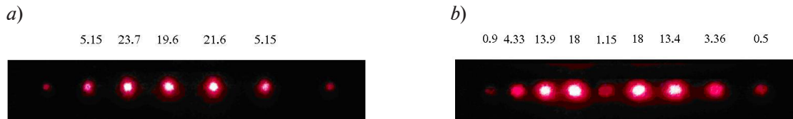
Fig. 7. Photographs of diffraction spectra for samples under normal incidence of illuminating laser beam, at spatial frequencies \nu = 212 \text{ mm}^{-1} ( a ) and 100 \text{ mm}^{-1} ( b ). The numbers above the diffraction spots indicate the DE values (in %)
