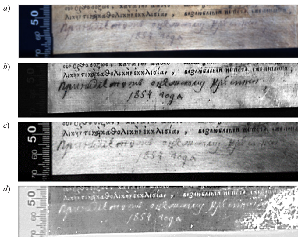
Fig. 2. Unreadable handwritten marginalia covered with restoration paper. Original (a); UV light, band 610 nm (b); halogen lamp, light band 570 nm (c) UV light, PCA-2 (d)
