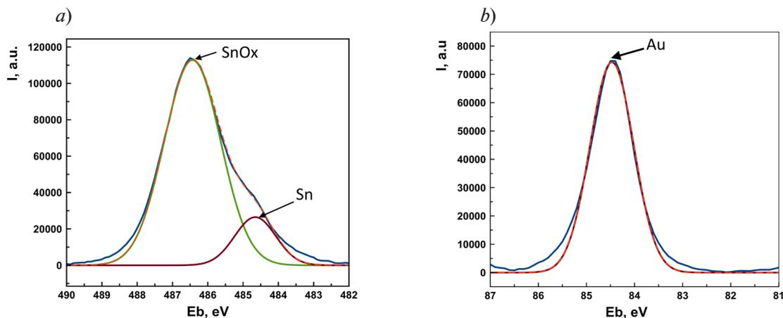
Fig. 3. XPS reference spectra of: Sn 3*d*<sub>5/2</sub> tin film with component decomposition (*a*); Au 4*f* gold film with component decomposition (each line corresponds to a spectrum component modeled using a Gaussian) (*b*)
