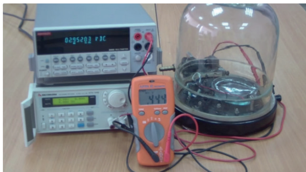
Fig. 2. Stand for measuring the output signal of the humidity sensor
