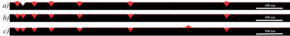
Fig. 4. Morphology of In droplet arrays obtained on patterned surfaces by means of the simulations at various temperatures: 250 °C ( a ), 200 °C ( b ) and 150 °C ( c )
