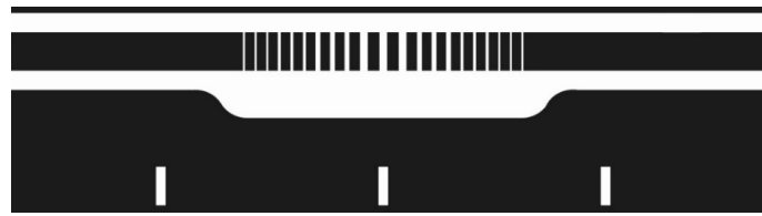
Fig. 2. Place where the storage chamber is combined with the mask of migration channels, 3 pieces of the same width (in microns) from left to right: 10, 15, 25, 50, 25, 15, 10
