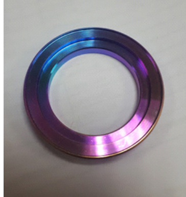
Fig. 5. Steel ring after atomic layer deposition
