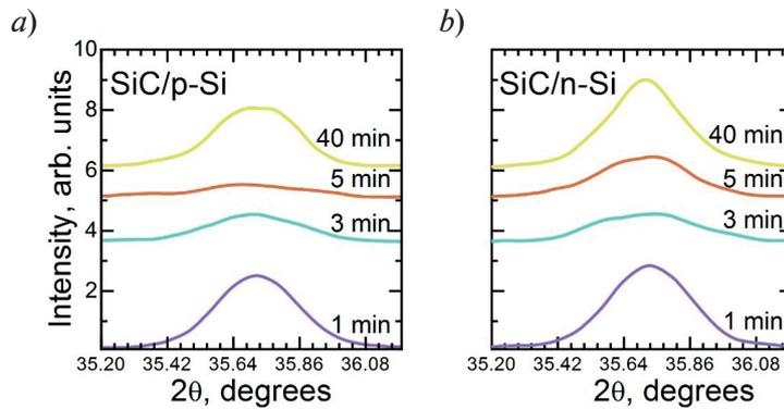
Fig. 2. XRD  $\omega - 2\theta$  spectra of the hybrid 3C-SiC(111)/Si(111) substrates at 3C-SiC(111) peak for the different growth times on (a) boron- and (b) phosphorus-doped silicon substrates obtained by DRON-8
