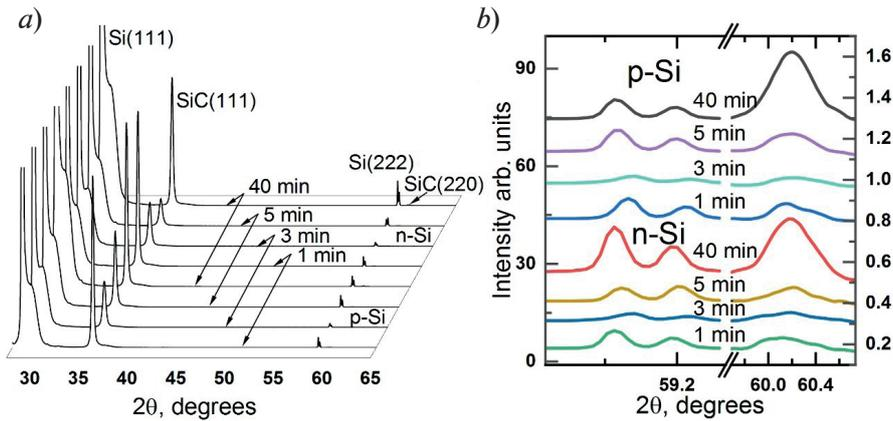
Fig. 1. XRD spectra of the 3C-SiC(111)/Si(111) substrates grown by the method of atomic substitution on *p*- and *n*-Si(111) substrates measured by Bruker advance d8 (a); the Si(222) and SiC(220) peaks from the spectra (b)
