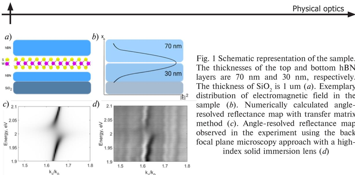
Fig. 1 Schematic representation of the sample. The thicknesses of the top and bottom hBN layers are 70 nm and 30 nm, respectively. The thickness of  $\text{SiO}_2$  is 1  $\mu\text{m}$  (a). Exemplary distribution of electromagnetic field in the sample (b). Numerically calculated angle-resolved reflectance map with transfer matrix method (c). Angle-resolved reflectance map observed in the experiment using the back-focal plane microscopy approach with a high-index solid immersion lens (d)
