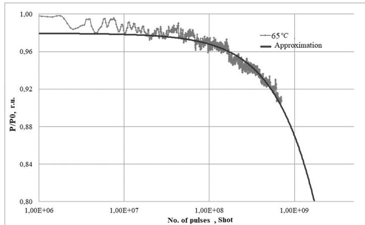
Fig. 2. The results of accelerated lifetime tests for LDA No. 1 at LDB junction temperature of 65 °C
