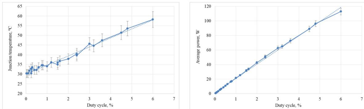
Fig. 1. Junction temperature and average radiation power vs. duty cycle
