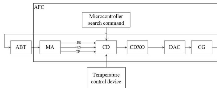
Fig. 2. Scheme of the AFC of the quantum frequency standard: ABT - atomic beam tube, MA - matching amplifier, CD - control device, QO - quartz oscillator, ES - error signal
