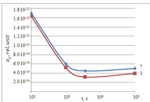
Fig. 4. Plot of the Allan variance  $\sigma_y$  versus time  $t$ . Graphs 1 and 2 correspond to the previously used AFC system in the QSC by us, respectively
