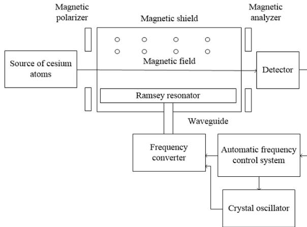
Fig. 1. The design of the cesium frequency standard
