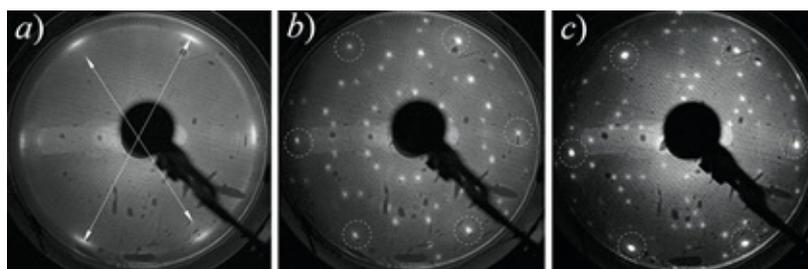
Fig. 3. LEED patterns (40 eV) for magnesium film Mg (0001) of 1.4 nm (a);  $\sqrt{7}\times\sqrt{7}$ -(Pb,Mg) (b);  $\sqrt{3}\times\sqrt{19}$ -(Pb,Mg) (c), dashed circles indicate the  $1\times 1$  spots.
