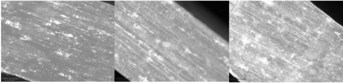
Fig. 1. The optical images of slices of the polyethylene films including diatomite; a filler content (% vol.) is 2 (left), 4 (in the center) and 6 (right)
