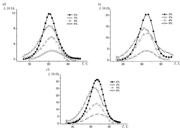
Fig. 5. Thermally stimulated depolarization spectra of the pure polyethylene films and of the composite polyethylene ones with diatomite. The heating rates (K/s) were  $5 \cdot 10^{-2}$  (a),  $1.0 \cdot 10^{-1}$  (b) and  $1.5 \cdot 10^{-1}$  (c).
