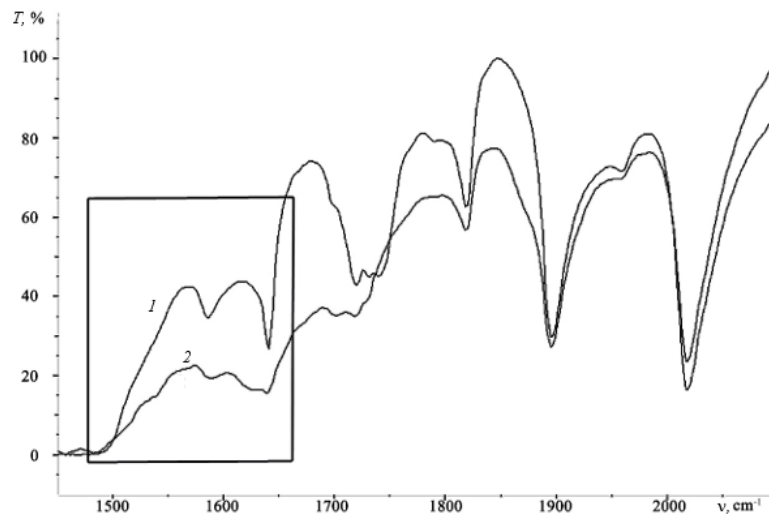
Fig. 2. IR transmission spectra of LDPE (1) and of the composite of LDPE + 6 % diatomite (2). The presence of water is highlighted
