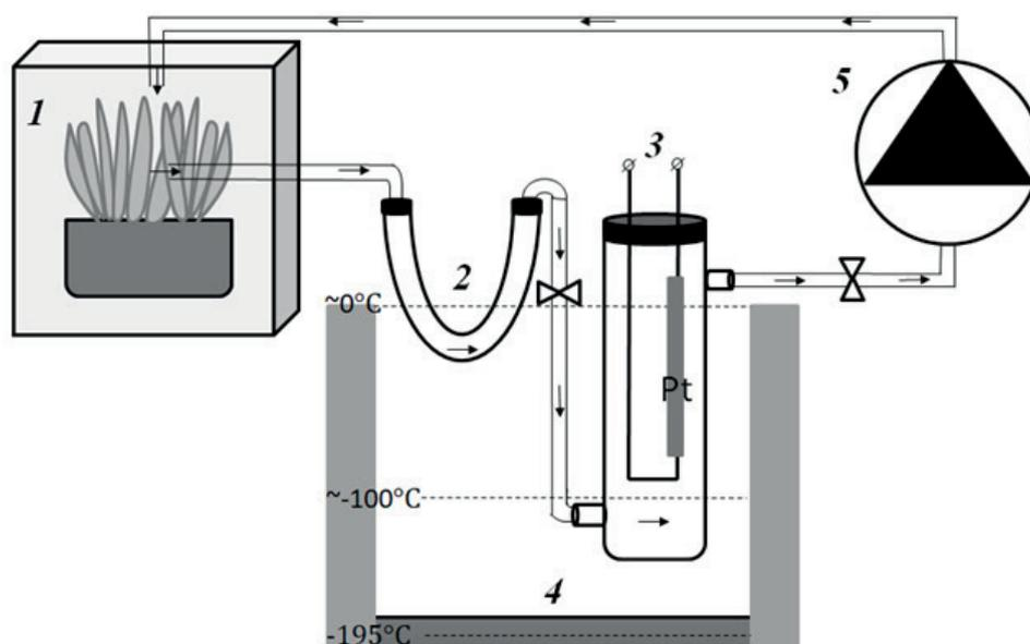
Fig. 1. Setup for enriching carbon dioxide from atmosphere surrounding the plant: sealed chamber *1* with air exhaust and supply pipes, U-shaped tube 2 for draining the gas mixture, Wurtz flask 3 for depositing carbon dioxide in nitrogen vapor with integrated catalytic chamber for afterburning organic impurities, heat-insulating vessel 4 with liquid nitrogen, flow controller 5 Temperature is controlled by a thermocouple
