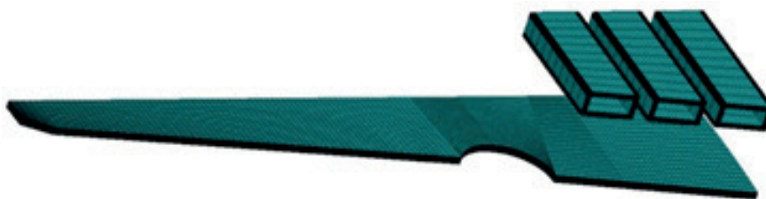
Fig. 2. Finite-element 3D system: induction coil 1, diaphragm spring 2
