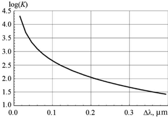
Fig. 4. The logarithm of the contrast intensity POS with zero order half-wave plate from the Gaussian width of the emission spectrum.  $\lambda_0 = 0.55 \mu\text{m}$ ,  $\Delta n_0 = 0.04$ ,  $l = 6.88 \mu\text{m}$
