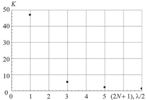
Fig. 5. The dependence of the contrast of the half-wave BF plate from created a path difference of the ordinary and extraordinary waves  $\Delta n_0 = 0.04$ , the Gaussian spectrum  $\lambda_0 = 0.55 \mu\text{m}$ ,  $\sigma = 0.05 \mu\text{m}$
