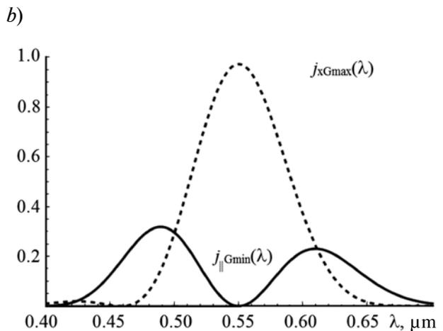
Fig. 6. The spectral density of white Gaussian light spectrum after passing  $\text{POS}_{x||}$  with a half-wave plate: a – zero-order ( $N = 0$ )  $\Delta n_0 = 0.04$ , thickness  $l = 6.88 \mu\text{m}$  ( $\lambda_0 = 0.55 \mu\text{m}$ ); b – after its passing  $\text{POS}_{x||}$  with a half-wave plate of second order ( $N = 2$ ),  $\Delta n_0 = 0.04$ , thickness  $l = 34.38 \mu\text{m}$
